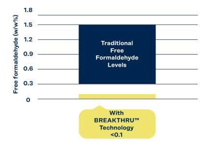
Effect on Free Formaldehyde Levels with BREAKTHRU™ Technology from Bakelite Synthetics
